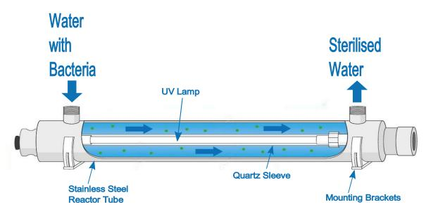
The glass quartz sleeve holds the UV lamp and protects it from direct contact with the water. It is transparent to the UV wavelength, which allows UV light to penetrate the glass and disinfect the water. A couple of o-rings hold it in place and prevent leakage.
